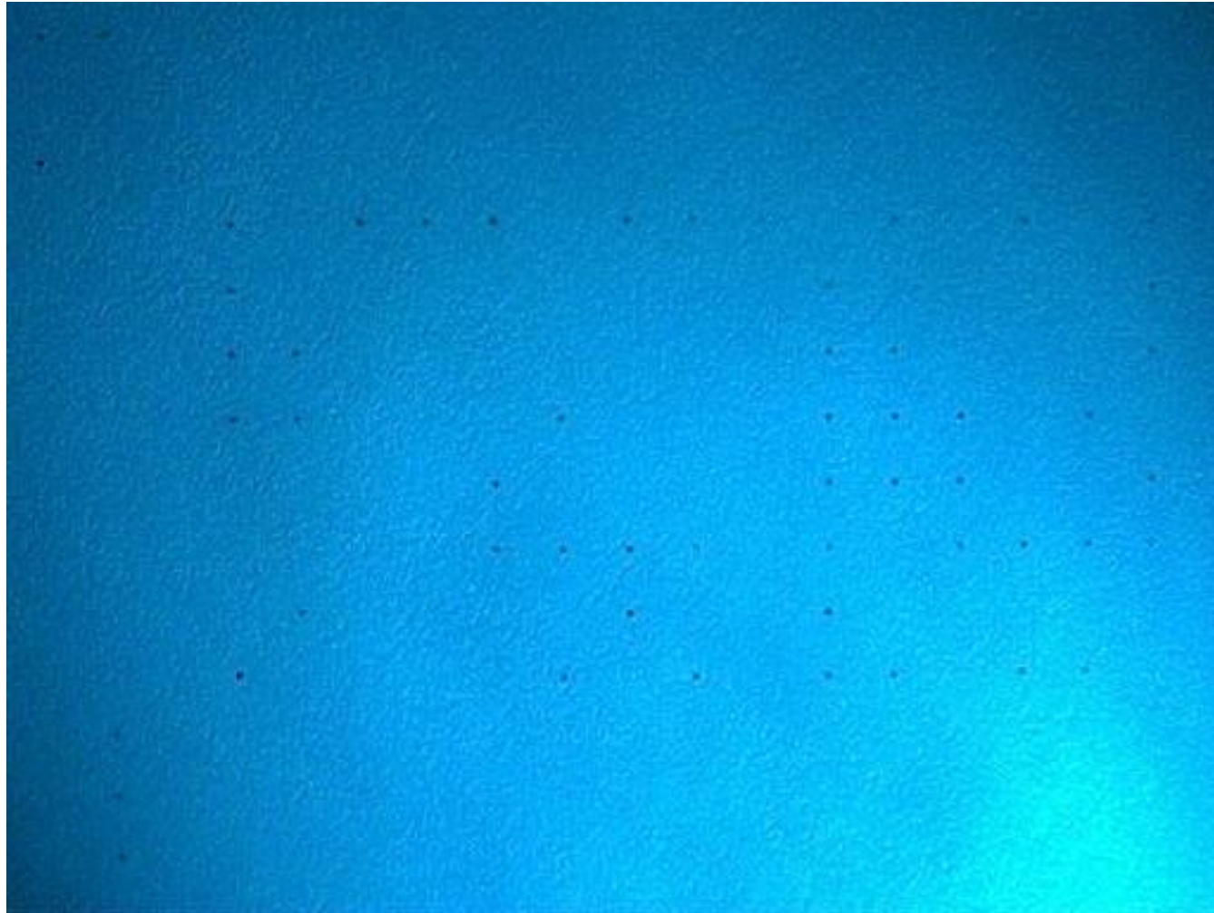
Xerox DocuColor 12 page, magnified 10x and photographed by the QX5 microscope under illumination from a Photon blue LED flashlight
